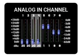
The GAINS display is used to adjust the sensitivity of the analog inputs. These are individually adjustable in 1dB steps from +20dBu to -8dBu. The number given below the fader indicates the maximum level that the converter accepts. If, for example, a fader is set to a value of 19, the input can process a level of 19 dBu maximum and in this case would output 0 dBFS on the digital side. Higher values would lead to
