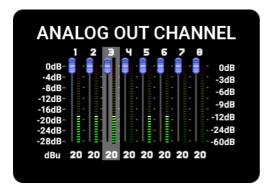
The LEVELS display is similar to the GAINS display and is used to adjust the output volumes. The outputs are also individually adjustable in 1 dB steps from +20dBu to -8dBu. Note that the levelmeter display does not change while you adjust, as the levels are shown before the attenuation is done.
