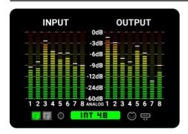
In the upper area the levels of the 8 inputs and 8 outputs are shown. As already described, you should absolutely avoid clipping, and therefore for example control the level only up to -6dB. Any clipping that may occur is indicated by a flashing bar at the top and can be deleted by briefly pressing the POWER button.
